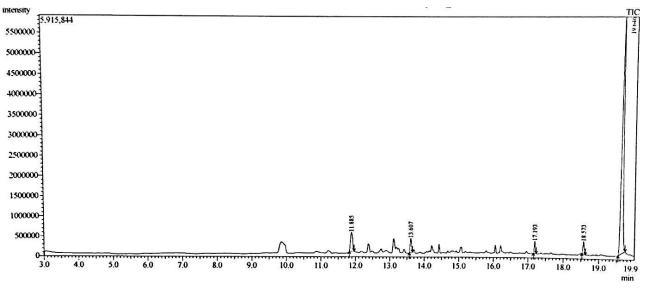
Figure 4. GC-MS chromatogram of EAF2
